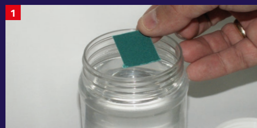
A dry swatch is placed on the surface of pure water.
