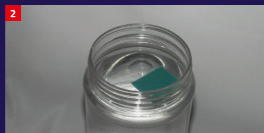
The pure water does not soak the swatch, the top of the swatch remains dry.
