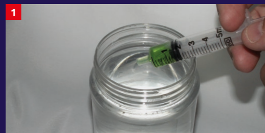
Class A foaming agent is added to the water at the proportioning rate recommended by the manufacturer.
