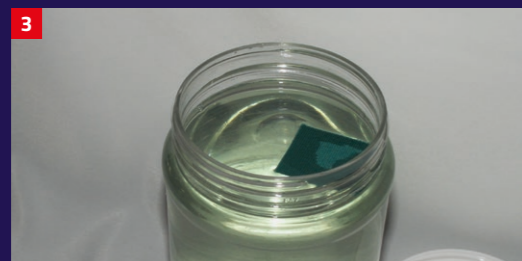
The water-foam concentrate mixture immediately penetrates and soaks the material.
